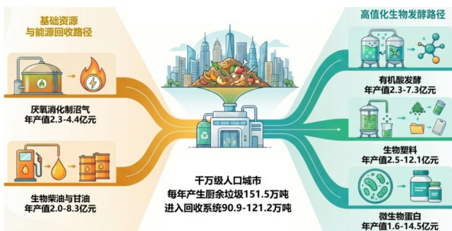
(c) 面向厨余垃圾, 构建以能源回收 (如沼气) 与高值化生物发酵 (如有机酸、PHA 及微生物蛋白) 为核心的多路径资源化体系 (c) For food waste, a multi-pathway resource utilization system is envisaged, centered on energy recovery (e.g., biogas) and value-added biofermentation (e.g., organic acids, PHA, and microbial protein)
